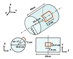
Figure 4 Phantom and coil geometry for DGF simulations in Figs. 5 to 9. The EM field associated with the coil (in orange) was calculated for the transverse plane through the center of the coil shown by the dotted line in the Y–Z plane. The shape of the coil is a cylindrical window that follows the curvature of the object.
