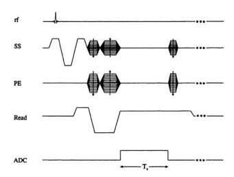
**Fig 1.** Gradient-echo sequence design.  $T_s$  refers to the sampling time interval. The gradient pulses are designed to give first-order flow compensation. SS indicates the slice-select gradient; PE, the phase-encoding gradient; ADC, analog-to-digital conversion.
