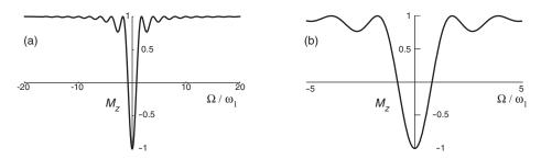
Fig. 3.28 Plots of the *z*-magnetization produced by a pulse as a function of the offset; the flip angle on-resonance has been set to 180°. Plot (b) covers a narrower range of offsets than plot (a). These plots should be compared with those in Fig. 3.26.
