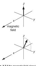
**Fig. 3.7** If the magnetic field along the *z* axis is replaced quickly by one along *x*, the magnetization will then precess about the *x* axis and so move towards the transverse plane.
