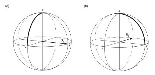
**Fig. 3.22** Grapefruit plots showing the effect on equilibrium magnetization of (a) a 90° pulse about the *y* axis and (b) a 90° pulse about the -x axis. Note the position of the  $B_1$  field in each case.
