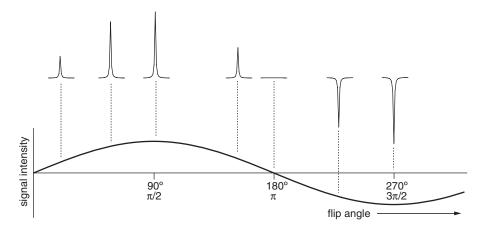
**Fig. 3.18** Illustration of how pulse calibration is achieved. The signal intensity varies as  $(\sin \beta)$  as shown by the curve at the bottom of the picture. Along the top are the spectra which would be expected for various different flip angles (indicated by the dashed lines). The signal is a maximum for a flip angle of 90° and goes through a null at 180°; after that, the signal goes negative.
