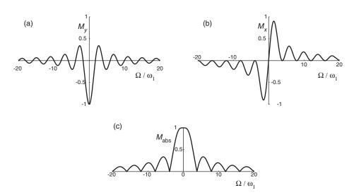
**Fig. 3.26** Plots of the magnetization produced by a pulse as a function of the offset. The pulse length has been adjusted so that on resonance the flip angle is 90°. The horizontal axes of the plots is the offset expressed as a ratio of the RF field strength,  $\omega_1$ ; the equilibrium magnetization has been assumed to be of size 1.
