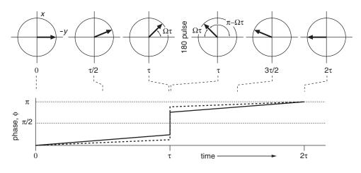
Fig. 3.19 Vector diagrams showing how a spin echo refocuses the evolution of the offset; see text for details. Also shown is a phase evolution diagram for two different offsets (the solid and the dashed line).
