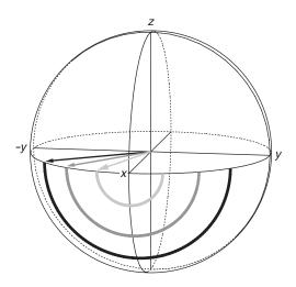
**Fig. 3.21** Illustration of the effect of a 180° pulse on three vectors which start out at different angles from the -y axis (coloured in black, grey and light grey). All three are rotated by 180° about the *x* axis on the trajectories indicated by the thick lines which dip into the southern hemisphere. As a result, the vectors end up in mirror image positions with respect to the *xz*-plane.
