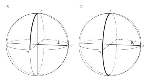
Fig. 3.12 A "grapefruit" diagram in which the thick line shows the motion of a magnetization vector during an on-resonance pulse. The magnetization is assumed to start out along +z. In (a) the pulse flip angle is 90°. The effective field lies along the x axis and so the magnetization precesses in the yz-plane. The rotation is in the positive sense about x so the magnetization moves toward the -y axis. In (b) the pulse flip angle is 180° and so the magnetization ends up along -z.
