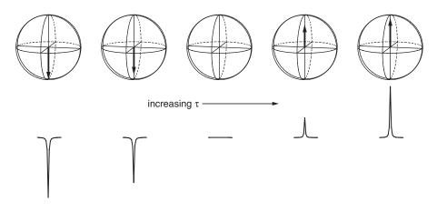
**Fig. 3.24** Visualization of the outcome of an inversion recovery experiment. The size and sign of the *z*-magnetization is reflected in the spectra (shown underneath). By analysing the peak heights as a function of the delay  $\tau$  it is possible to find the rate of recovery of the *z*-magnetization.
