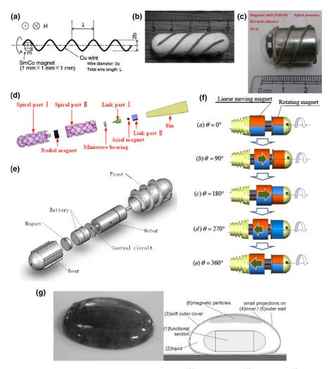
Fig. 6. Spiral and Hybrid Capsule Designs: (a) First reported spiral robot, Honda et al. (b) Chiba et al., (c) Bo et al., (d) Guo et al., (e) Wang et al., (f) Yim et al., (g) Magnetically controlled crawling movement by Nokata et al. (eft) soft model prototype for crawling in an uneven surface, (right) structure of a rolling object using magnetic derive principle with sample magnetic field. [Color figure can be viewed at wileyonlinelibrary.com]
