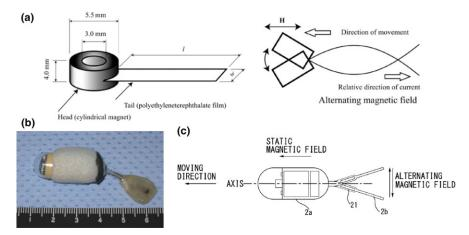
Fig. 5. (a) Magnetic swimming mechanism by use of alternating magnetic fields and a flexible tail by Sudo et al. <sup>128</sup> (b) Capsule with permanent magnet in a fin by Morita et al. <sup>132</sup> (c) Schematic from patent filing showing fish-like robot. <sup>135</sup> [Color figure can be viewed at wileyonlinelibrary.com]
