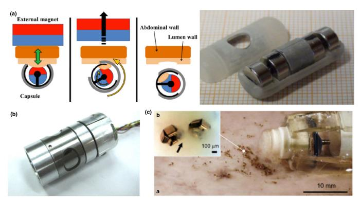
Fig. 7. Biopsy sampling capsules: (a) Mechanism of tissue retrieval developed by Simi et al., <sup>181</sup> (b) Capsule with rotary blades released using shape memory alloys by Kong et al., <sup>182</sup> (c) Deployment of magnetic microgrippers for biopsy sampling by Yim et al. <sup>183</sup> [Color figure can be viewed at wileyonlinelibrary.com]
