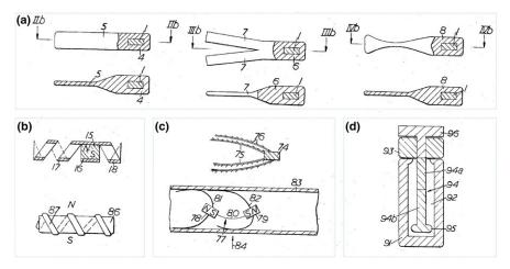
Fig. 3. A selection of devices for magnetic propulsion adapted from the patent application of Frei and Leibinzhon:<sup>59</sup> (a) Endorobots with single or multiple tails.<sup>33</sup> (b) Screw-like robots which are transversely magnetized and can propel longitudinally forward. (c) Robots for swimming inside tubes by utilizing surface friction. (d) Robot for propulsion and drug release.
