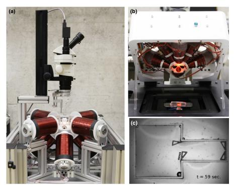
Fig. 8. (a) OctoMag with eight electromagnetic coils. (b) Nanomag electromagnet system mounted on an inverted microscope. (c) RodBot pushing and assembling triangle-shaped micro-objects. [Color figure can be viewed at wileyonlinelibrary.com]
